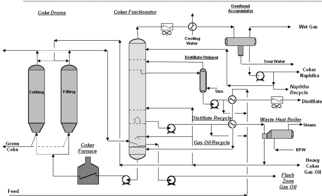
Figure 1; Typical Basic Process Flow Diagram of a Delayed Coker Unit (Schematic provided by Bechtel Hydrocarbon Technology Solutions, Inc.)
