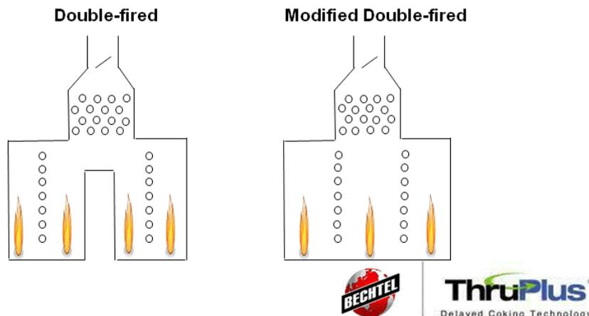
Figure 2; One Cell of a Double Fired and Modified Double Fired Furnace
